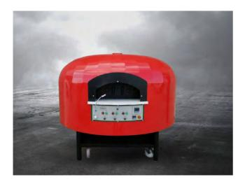
In Maximum series ovens, the below stone thickness is 5 centimeters. Since the stone was heated from below, we preferred 5 centimeters, which is the ideal thickness. It passes the heat fast to the upper surface during combustion and a suitable thickness for heat storage. Under the cooking stone, there is a burner that operates with a thermostat. This burner heats the stone faster and transfers extra heat to the firing section of the oven.
